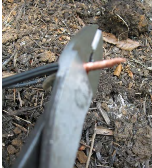
Step 2 - Crimp Copper Barrel on Wire
